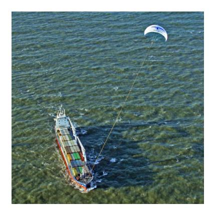
Real wind power: Long-distance cargo ships burn large amounts of fuel and contribute to air pollution. One German shipping company is experimenting with special kites to help reduce both problems. The big kite helps to pull the ship so the ship's engines will burn less fuel every day. As they burn less fuel, the amount of air pollution the engines produce will also be reduced.
