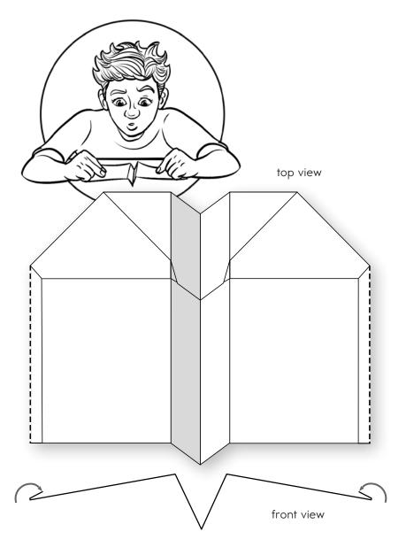
Next, fold the outside edge of each wing up about a finger's width.
